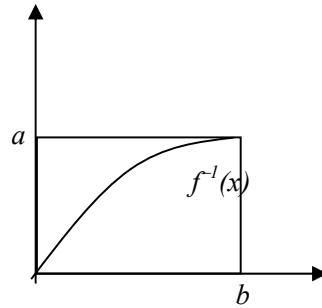
From the diagram, it's clear that the area under the curve of  $f(x)$  + the area under the curve of  $f^{-1}(x)$  is the area of the rectangle.
